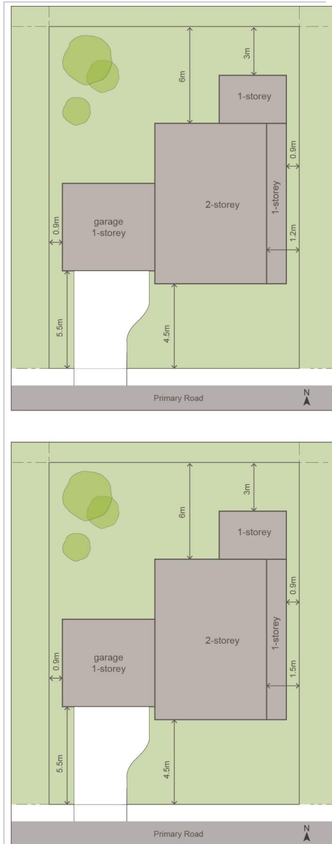
Figure 2: Setback Controls (lot located outside the FSPA above, lot located within FSPA below)
