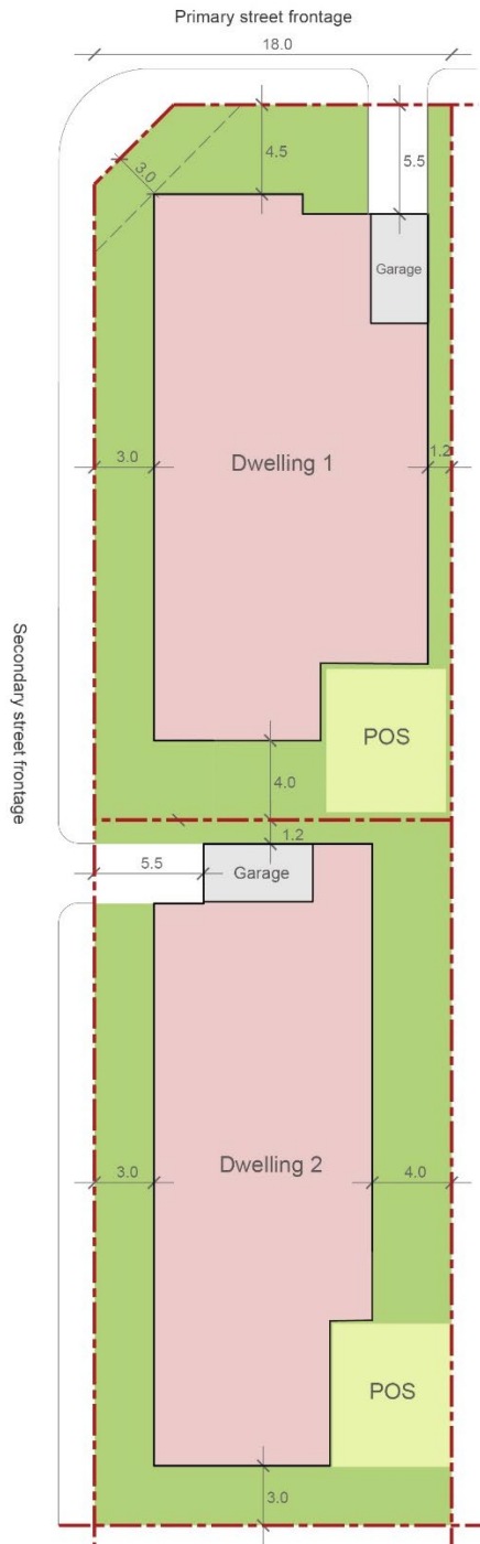
Figure 5: Detached dual occupancy - Corner site (dual frontage). Note: all dimensions are in metres.
