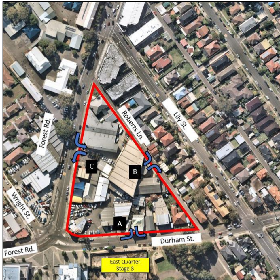
Figure 11: Recommended Vehicular Access Points
