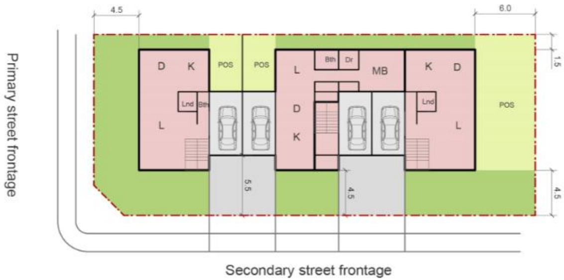
Figure 5: Manor House (dual frontage)
