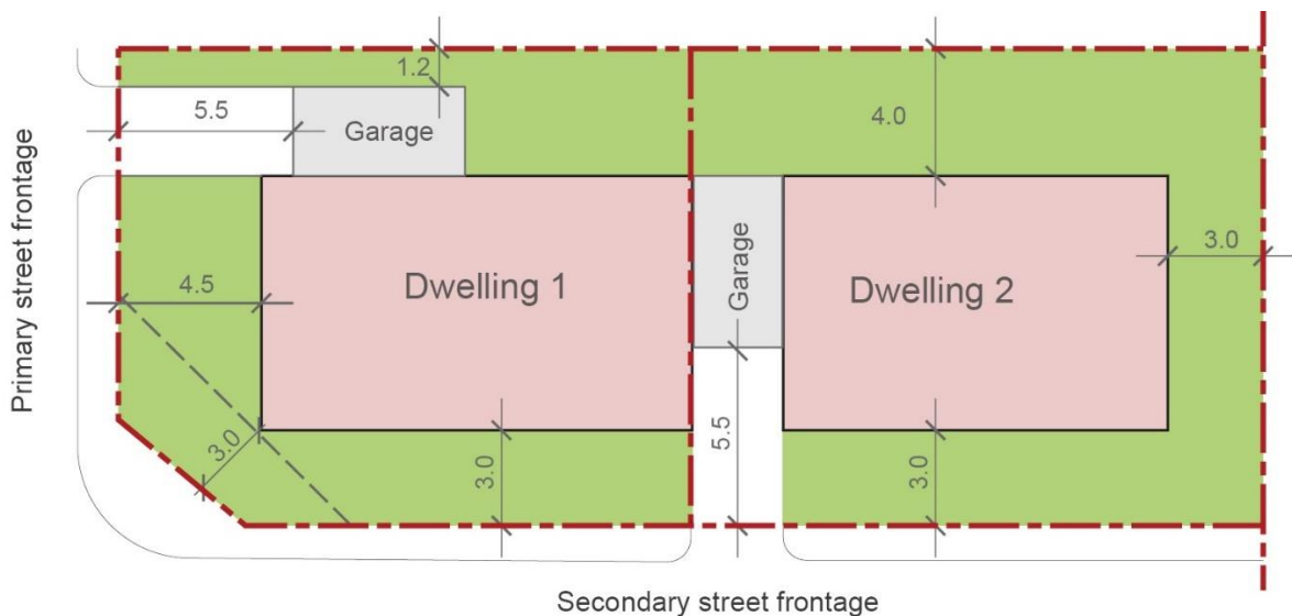
Figure 9: Attached dual occupancy – Corner Site (dual frontage). Note: all dimensions are in metres.
