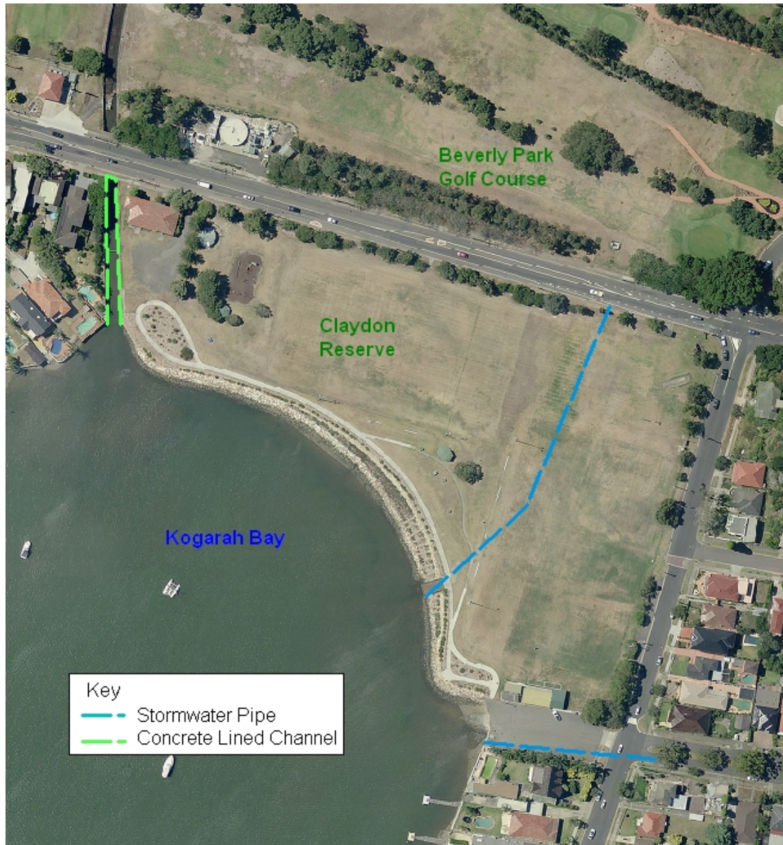
Figure C.4 Stormwater Pipe Layout
