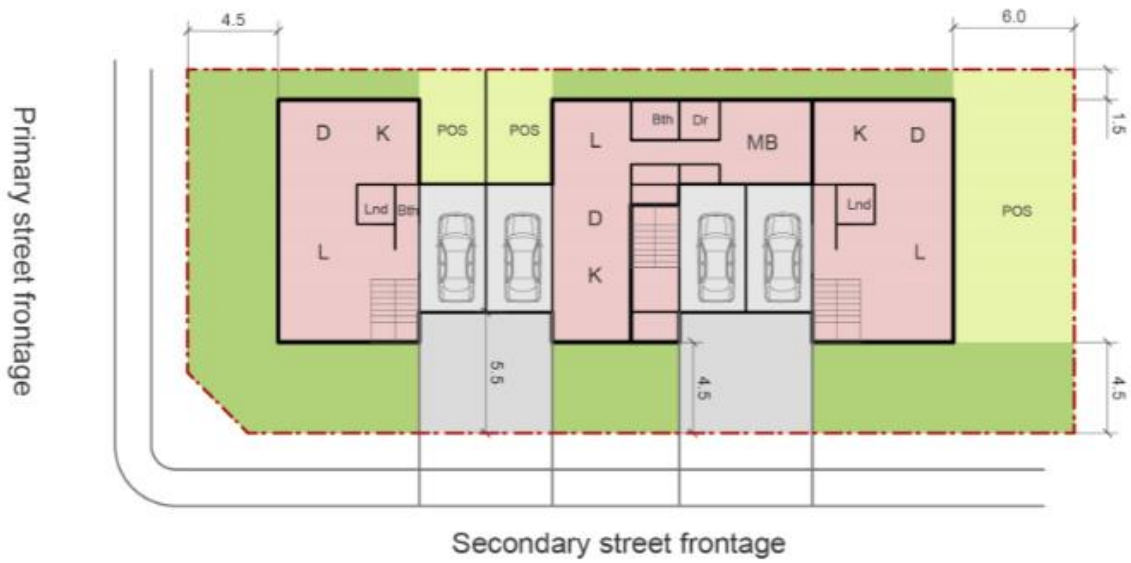
Figure 5: Manor House (dual frontage)
