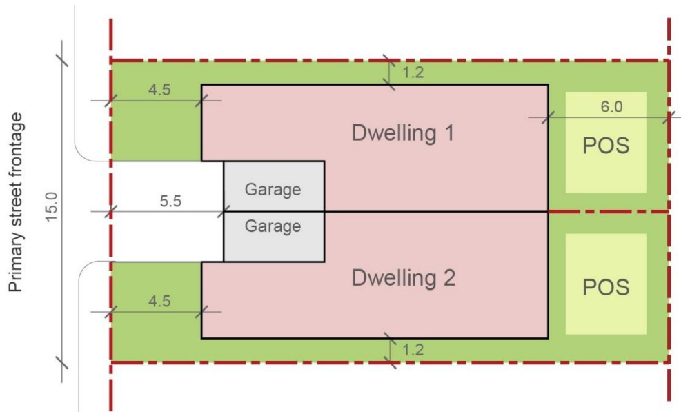
Figure 55: Attached dual occupancy in a 'side by side' configuration. Note: all dimensions are in metres
