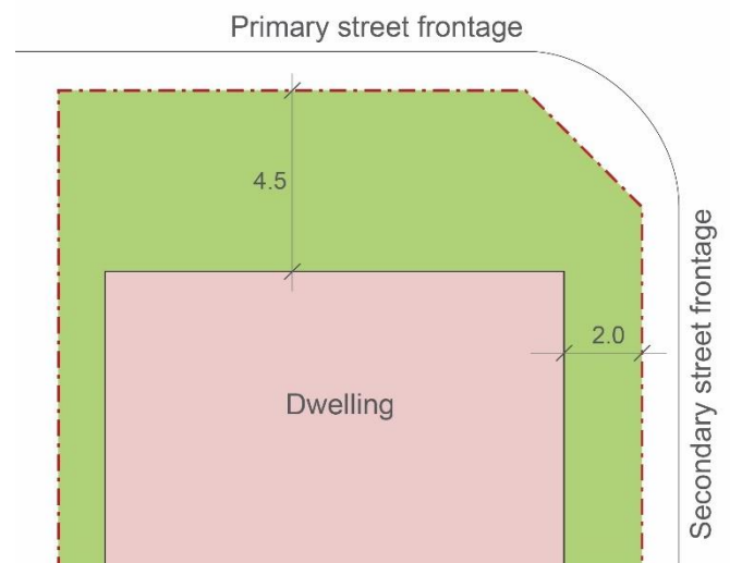
Figure 22: Setback from secondary street boundary for sites 15m or greater in width
