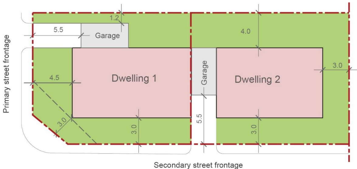
Figure 99: Attached dual occupancy – Corner Site (dual frontage). Note: all dimensions are in metres.
